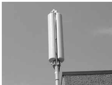
The MSO24014PTNF's mount design allows mast or tower leg mounting for greater flexibility when tower space availability is limited.
