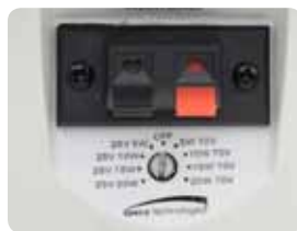
Transformer Dial & Terminals
