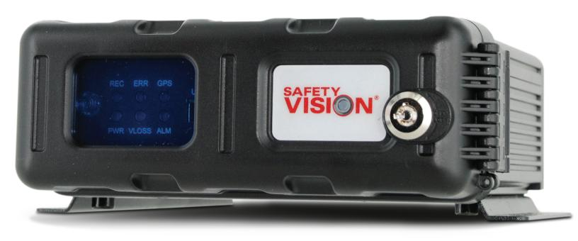
The Observer™ 4000 HYB hybrid video recorder (HVR) is designed with the specialized capability to work with analog and high definition cameras simultaneously. Four Analog High Definition (AHD) connections support up to 720p HD resolution utilizing traditional analog cables, plus an additional Ethernet connection supports a fifth IP camera with a resolution up to 1080p. Generate amazing HD images at an analog price with dependable performance that has made the Observer series an industry leader.
