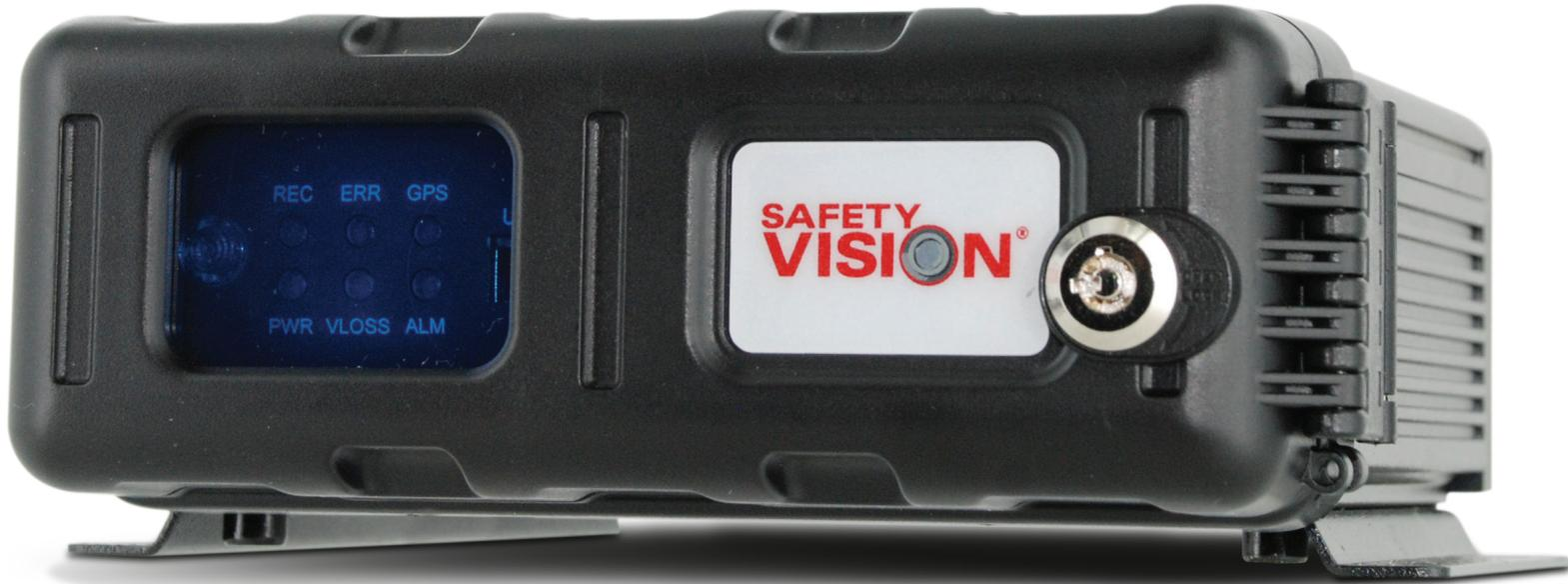
The Observer™ 4000 HYB hybrid video recorder (HVR) is designed with the specialized capability to work with analog and high definition cameras simultaneously. Four Analog High Definition (AHD) connections support up to 720p HD resolution utilizing traditional analog cables, plus an additional Ethernet connection supports a fifth IP camera with a resolution up to 1080p. Generate amazing HD images at an analog price with dependable performance that has made the Observer series an industry leader.
